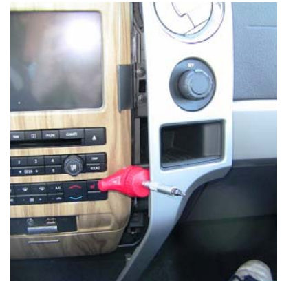
Showing method of holding open bezel to install mount.
